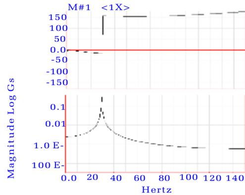
Figure 5B Bode plot of same pure 30 hertz sine wave, but with a 90 degree phase shift compared to Figure 5A.
