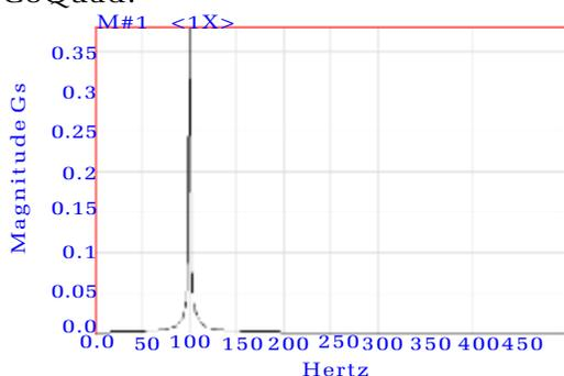
Figure 6C Standard autospectrum display of 100 hz signal.
