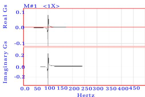
Figure 6A Real and imaginary portions of a 100 hz signal, this format is sometimes referred to as CoQuad.
