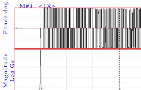
Figure 7A CoQuad display of complex spectrum with minimal leakage
