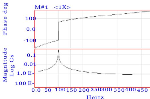
Figure 6B Bode plot of the same signal. Note that the amplitude scale for the bode plot is logarithmic.
