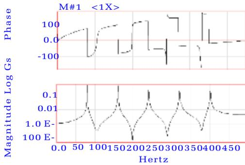
Figure 5C Bode plot depiction of complex spectrum with 5 different individual frequency components.
