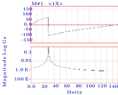
Figure 5A Bode plot of a pure 30 hertz sine wave with 70 degrees phase at 30 Hz.
