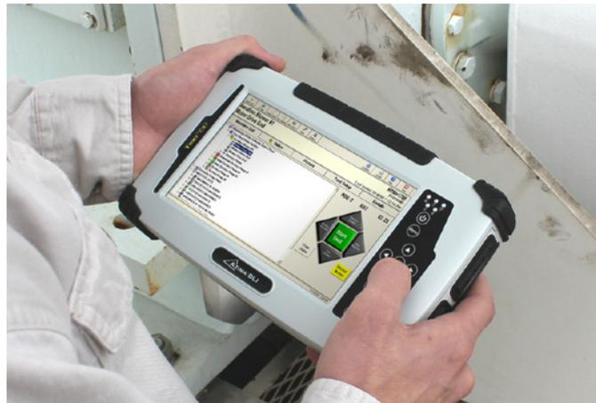
Figure 1: Vibration Analyst using diagnostic software for CBM program
