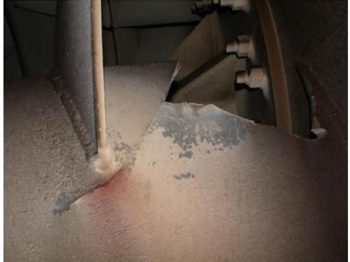
Azima DLI quickly deployed its Roamer (a mobile remote monitoring system) and began taking data every 10 minutes. Within one day, the Azima DLI analyst determined that running the fan at 90% speed would reduce the stress on the blade, but not impact production. The mill made the speed change and Azima DLI continued to collect data at 10-minute intervals. If the situation worsened, the Azima DLI diagnostic system would alert the analyst and mill staff immediately.
