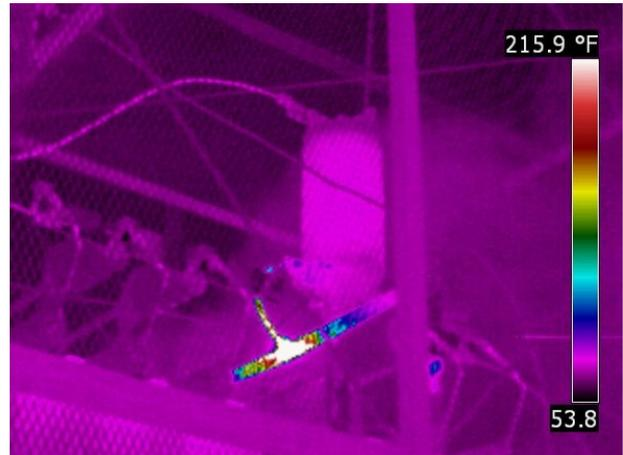
A potentially catastrophic electrical fault was discovered at Total Petrochemicals during a routine annual infrared thermography survey performed by Azima DLI. The reactor appeared to be operating normally but the infrared inspection revealed a faulty wire connection and critical heat damage to the aluminum bus bar that would otherwise have gone undetected until failure.
