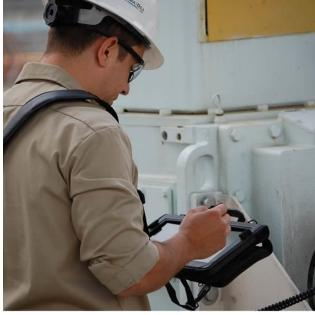
With today's versatile and portable data collection systems, you are basically doing EKG's on machines. Just like when you go to the doctor, an EKG will detect any early problems. Similarly, machines will give off precursors, or early indicators, of future problems when using this type of solution.
